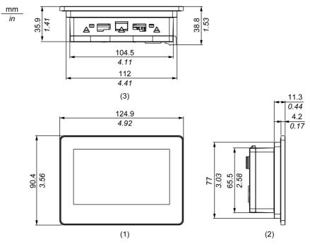
NOTE: External view is shown using first angle projection method.
