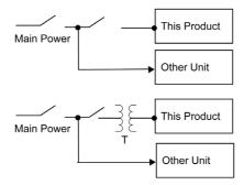
• Use SELV (Safety Extra-Low Voltage) circuit and LIM (Limited Energy circuit) for DC power.
